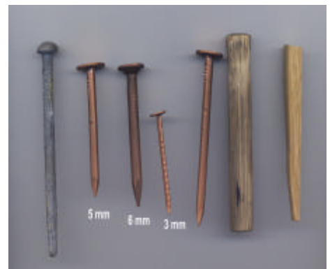
Figure 25. Many different pegs and nails have been used to fix stone-slates over the years. Stout copper nails or pegs are preferred for strength and durability.
