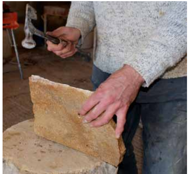
Hand dressing Cotswold slates at Down Ampney delph
